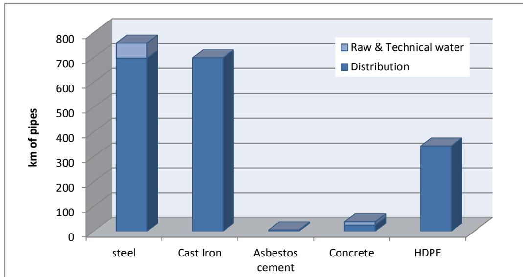
**Figure 8: Pipe Materials within the Distribution Network**
