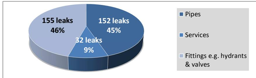
Figure 29: Number and Location of Leaks Detected within the Pilot leakage Study
